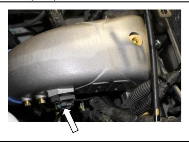
18. Tighten intake to boot connection with the supplied clamp. Tighten until spring is bound. (13mm)
