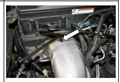
17. Apply some dielectric grease to the MAP sensor connector and reconnect the MAP sensor.
