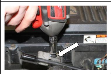
Loosen clamp between the rubber boot and the intake horn. Use a blade screwdriver to gently break the seal. (11mm)
