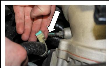
**NOTE:** Early models (2007.5-2009) will need to disconnect the exhaust temperature sensor at the rear of the intake horn.
