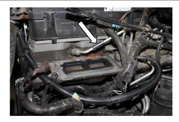
Disconnect the outlet Boot from the CAC (Drivers side) and pull out the pipe with boot and OEM clamp. (11mm)
