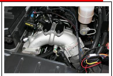
2. Remove the bolt holding the dipstick to the intake horn. (10mm socket)
