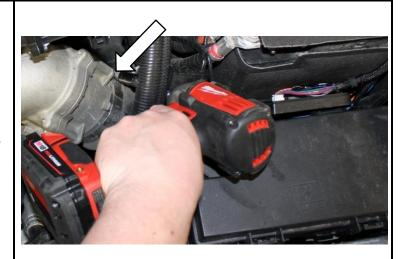
4. Pull off the harness clip from the intake horn.
